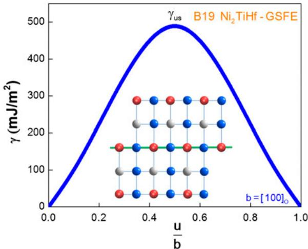
Figure 16. (colour online) The GSFE curve of the slip system  $(001)[100]$  in B19  $\text{Ni}_2\text{TiHf}$ . The calculated unstable SFE  $\gamma_{us}$  is given in Table 2.
