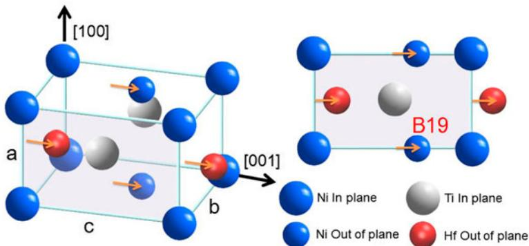
Figure 9. (colour online) The basal shuffle mode  $(0\ 1\ 0)[0\ 0\ 1]$  in B19 Ni<sub>2</sub>TiHf, i.e. atoms in  $(0\ 1\ 0)$  plane move in the  $[0\ 0\ 1]$  direction.
