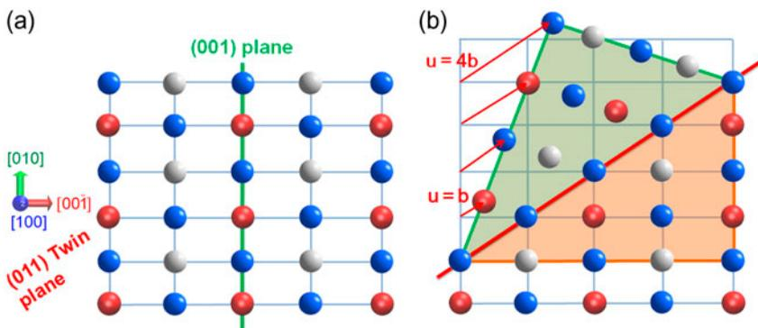
Figure 11. (colour online) Schematic of twinning in the  $(0\ 1\ 1)$  plane with dislocation  $[0\ 1\ \bar{1}]$  of B19  $\text{Ni}_2\text{TiHf}$ . (a) The perfect B19 lattice observed from the  $[1\ 0\ 0]$  direction. The twin plane  $(0\ 1\ 1)$  is marked with a red line and the  $(0\ 0\ 1)$  symmetry plane shown in green line is the plane of symmetry. (b) The lattice with a four-layer twin after shearing  $4b$  ( $b = \frac{1}{18}[0\ 1\ \bar{1}]$ ) shown in a red arrow.
