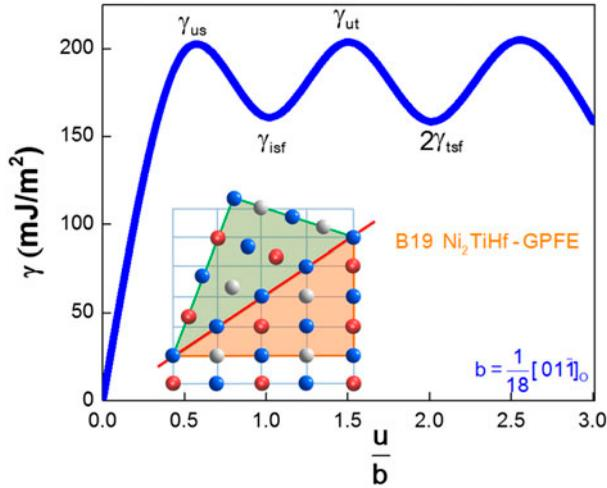
Figure 12. (colour online) The GPFE curve in  $(011)$  twin plane with  $[01\bar{1}]$  twinning dislocation of B19  $\text{Ni}_2\text{TiHf}$ . The shear displacement,  $u$ , is normalized by the twinning Burgers vector  $b = \frac{1}{18}[01\bar{1}]$ . The calculated fault energies are given in Table 2.
