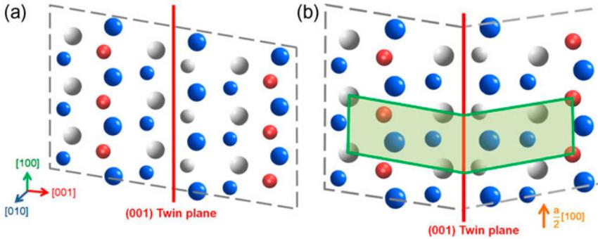
Figure 5. (colour online) Schematic of twinning in the (001) plane with twinning dislocation  $\frac{1}{2}[100]$  of  $B19'$   $Ni_4Ti_3Hf$ . (a) The perfect  $B19'$  lattice observed from the [010] direction. The twin plane (001) is marked with a red line. (b) The lattice with a two-layer twin after shearing along  $\frac{1}{2}[100]$  shown in a brown arrow.
