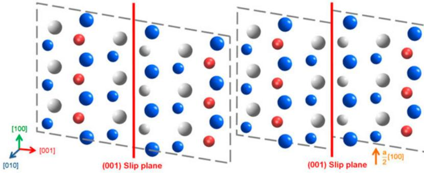
Figure 7. (colour online) Schematic of slip in the (001) plane with dislocation  $\frac{1}{2}[100]$  of B19'  $\text{Ni}_4\text{Ti}_3\text{Hf}$ . (a) The perfect B19' lattice observed from the [010] direction. The slip plane (001) is marked with a red line. (b) The lattice after a rigid shear with dislocation  $\frac{1}{2}[100]$  is shown in a brown arrow.
