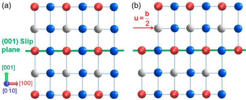
Figure 15. (colour online) Schematic of dislocation slip in the  $(001)$  plane with  $[100]$  dislocation of B19  $\text{Ni}_2\text{TiHf}$ . (a) The perfect B19 lattice observed from the  $[0\bar{1}0]$  direction. The slip plane  $(001)$  is marked with a green line. (b) The lattice after a rigid shear with displacement  $u = \frac{b}{2}$  ( $b = [100]$ ) shown in a red arrow.
