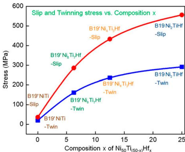
Figure 3. (colour online) Predicted dislocation slip and twinning stress in the martensite phase of  $\text{Ni}_{50}\text{Ti}_{(50-x)}\text{Hf}_x$  alloys, variation with composition  $x$  ( $x=0$ , NiTi;  $x=6.25$ ,  $\text{Ni}_8\text{Ti}_7\text{Hf}$ ;  $x=12.5$ ,  $\text{Ni}_4\text{Ti}_3\text{Hf}$ ;  $x=25$ ,  $\text{Ni}_2\text{TiHf}$ ). The stress values are given in Table 2.
