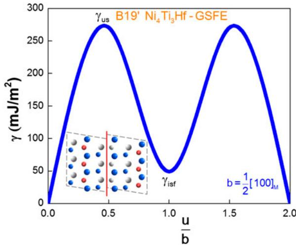
Figure 8. (colour online) The GSFE curve of the slip system (001)[100] in B19'  $\text{Ni}_4\text{Ti}_3\text{Hf}$ . The dislocation  $[100]$  can dissociate into two partials  $\frac{1}{2}[100]$  connected by a SFE  $\gamma_{\text{isf}}$ . The calculated  $\gamma_{\text{isf}}$  and unstable SFE  $\gamma_{\text{us}}$  are given in Table 2.
