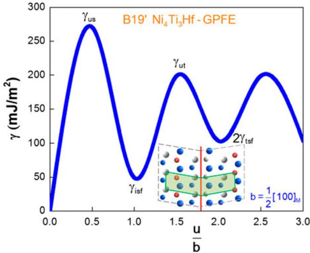
Figure 6. (colour online) The GPFE curve in the twin plane (001) with twin dislocation  $\frac{1}{2}[100]$  of  $B19'$   $Ni_4Ti_3Hf$ . The shear displacement,  $u$ , is normalized by the twinning Burgers vector  $b = \frac{a}{2} = 1.485 \text{ \AA}$ . The calculated fault energies are given in Table 2.
