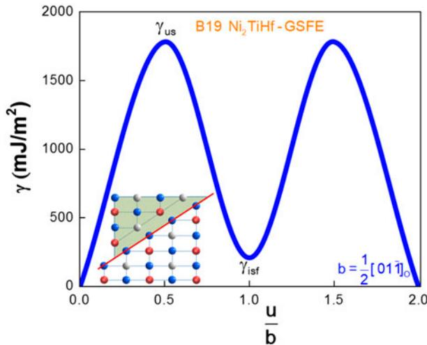
Figure 14. (colour online) The GSFE curve of the slip system (0 1 1)[0 1 1] in B19 Ni<sub>2</sub>TiHf. The dislocation  $[0 \bar{1} 1]$  can dissociate into two partials  $\frac{1}{2}[0 \bar{1} 1]$  connected by a SFE  $\gamma_{isf}$ . The calculated  $\gamma_{isf}$  and unstable SFE  $\gamma_{us}$  are given in Table 2.
