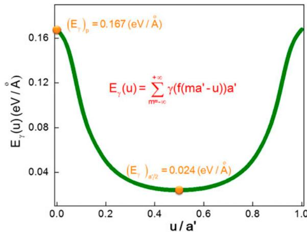
Figure 2. (colour online) Misfit energy  $E_\gamma(u)$  for the dislocation  $(011)[01\bar{1}]$  of B19 Ni<sub>2</sub>TiHf.
