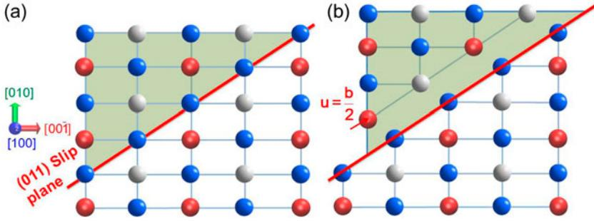
Figure 13. (colour online) Schematic of dislocation slip in the plane (0 1 1) with dislocation  $[0 \bar{1} 1]$  of B19 Ni<sub>2</sub>TiHf. (a) The perfect B19 lattice observed from the  $[1 0 0]$  direction. The slip plane (0 1 1) is marked with a red line. (b) The lattice after a rigid shear with displacement  $u = \frac{b}{2}$  ( $b = \frac{1}{2}[0 \bar{1} 1]$ ) shown in a red arrow.
