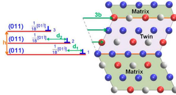
Figure 1. (colour online) Schematic of three-layer twin formation in B19 Ni<sub>2</sub>TiHf. The twin plane is (011) and twinning Burgers vector is  $\frac{1}{18}[01\bar{1}]$ ;  $h$  is the twin thickness and  $d_i$  is the equilibrium spacing between two adjacent twinning dislocations  $i$  and  $i+1$  corresponding to the minimum total energy. For the case of twin nucleation of B19 Ni<sub>2</sub>TiHf, we have  $i=1, 2$ .
