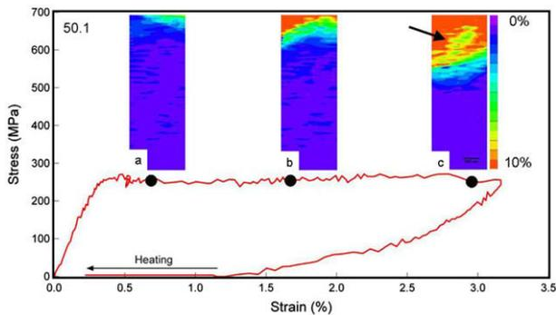
**Figure 2.** The nominal stress–strain curve, and the strain fields for Ti–50.1% Ni. The strain fields show the transformation front motion during increased deformation from points (a–c). The strain field is approximately 1.7 mm wide.
