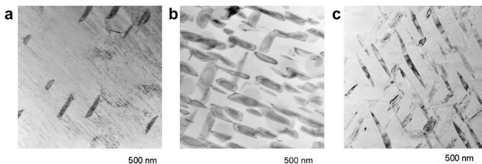
**Figure 1.** Transmission electron micrographs showing precipitate distribution for (a) Ti–50.1% Ni, (b) Ti–50.8% Ni, (c) Ti–51.5% Ni [4].
