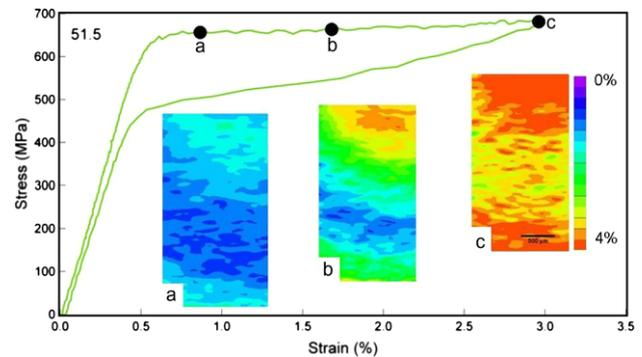
**Figure 4.** The nominal stress–strain curve, and the strain fields for Ti–51.5% Ni showing the transformation front motion during increased deformation from points (a–c). The strain field is approximately 1.4 mm wide.
