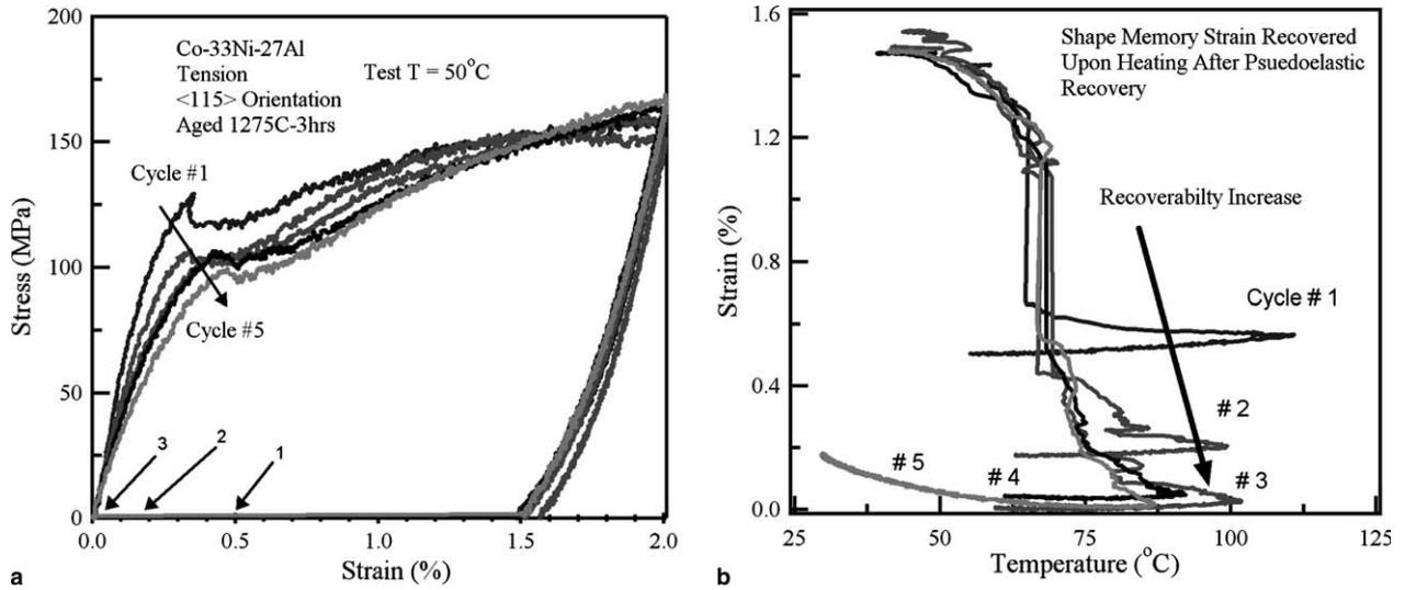
Fig. 6. (a) Stress–strain response at a test temperature of 50 °C showing an increase in recoverability near  $M_s$  from cycle #1 to #5 and (b) increasing shape memory strain recovery upon heating.
