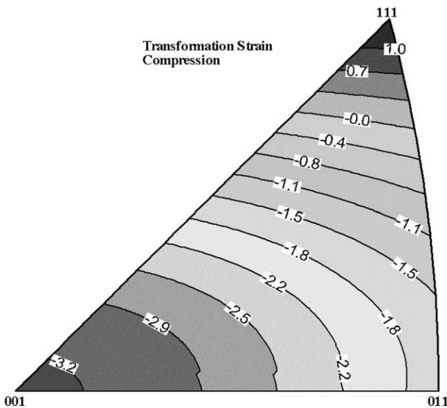
Fig. 9. Theoretical contours of transformation strain in compression. The contours for tension can be found in [7].
