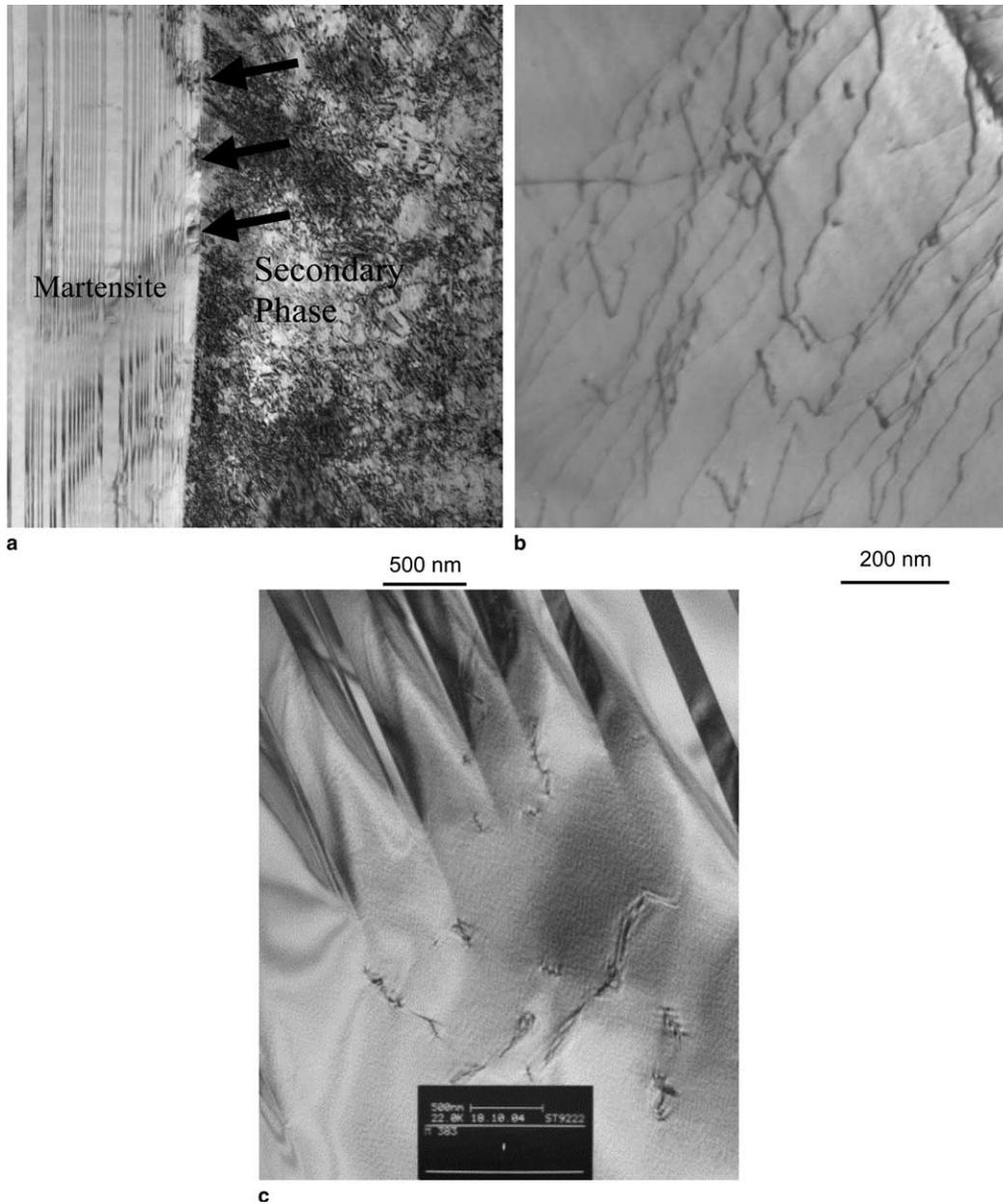
Fig. 3. (a) Transmission electron microscopy (TEM) bright field image of martensite next to a second phase boundary showing a high density dislocations in the second phase and arrows indicate that dislocations may be inherited by impinged martensite, (b) TEM bright field image of dislocations in the matrix phase and (c) Isolated dislocations in CoNiAl and the lamellar structure in the background is residual martensite.
