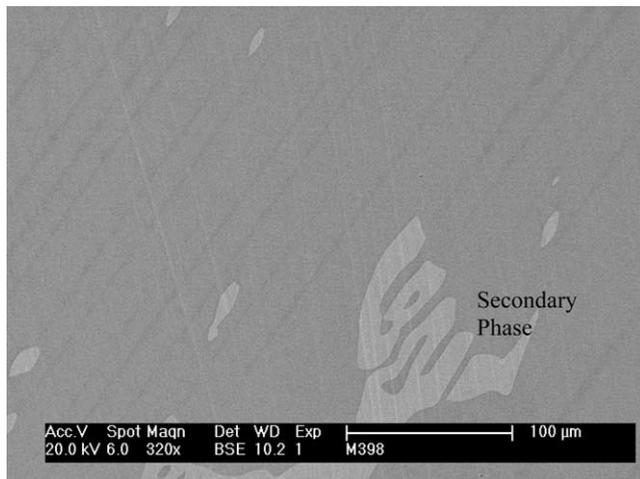
Fig. 2. Scanning electron microscope (SEM) image of the secondary phase in CoNiAl and the parallel dark thin bands are residual martensite plates. The martensite plates impinge on the second phase and in regions where the second phase is absent, the martensite growth proceeds uninhibited.
