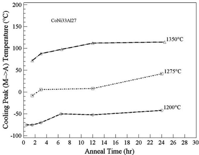
Fig. 1. Peak temperatures determined using differential scanning calorimetry (DSC) showing the forward transformation temperature variations as a function of annealing temperature and time.
