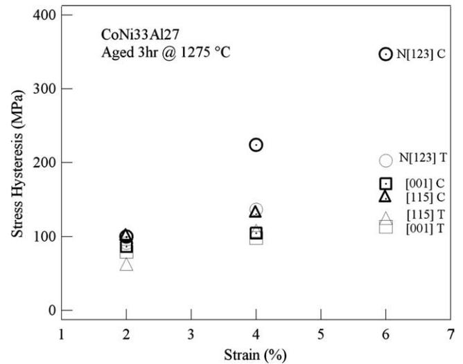
Fig. 10. Stress hysteresis in tension (T) and compression (C), bold shapes with centered dots, as obtained in experiments with incremental increase in strain. The stress hysteresis is determined from stress–strain curves shown in Fig. 8 at approximately half of the applied strain.
