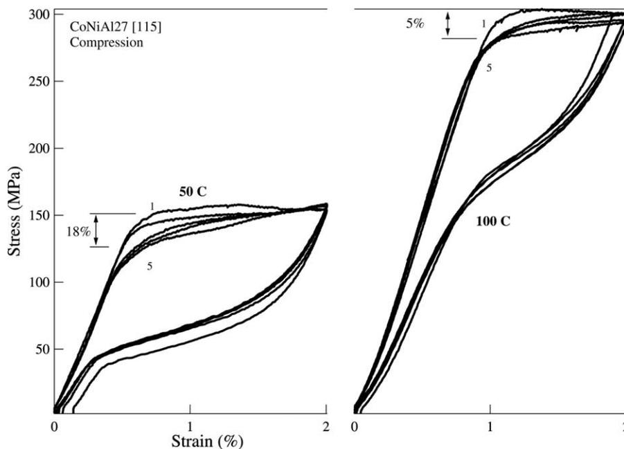
Fig. 5. Cyclic stress–strain curves of the [115] orientation under compression at 50 and 100 °C showing approximately 18% and 5% decrease in critical stress respectively.
